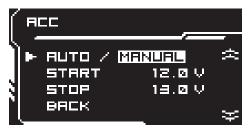
\* After powering on, navigate to ACC and select MANUAL. The system will then automatically switch on/off based on the input voltage. Please refer to "More Setting" on page 6.
